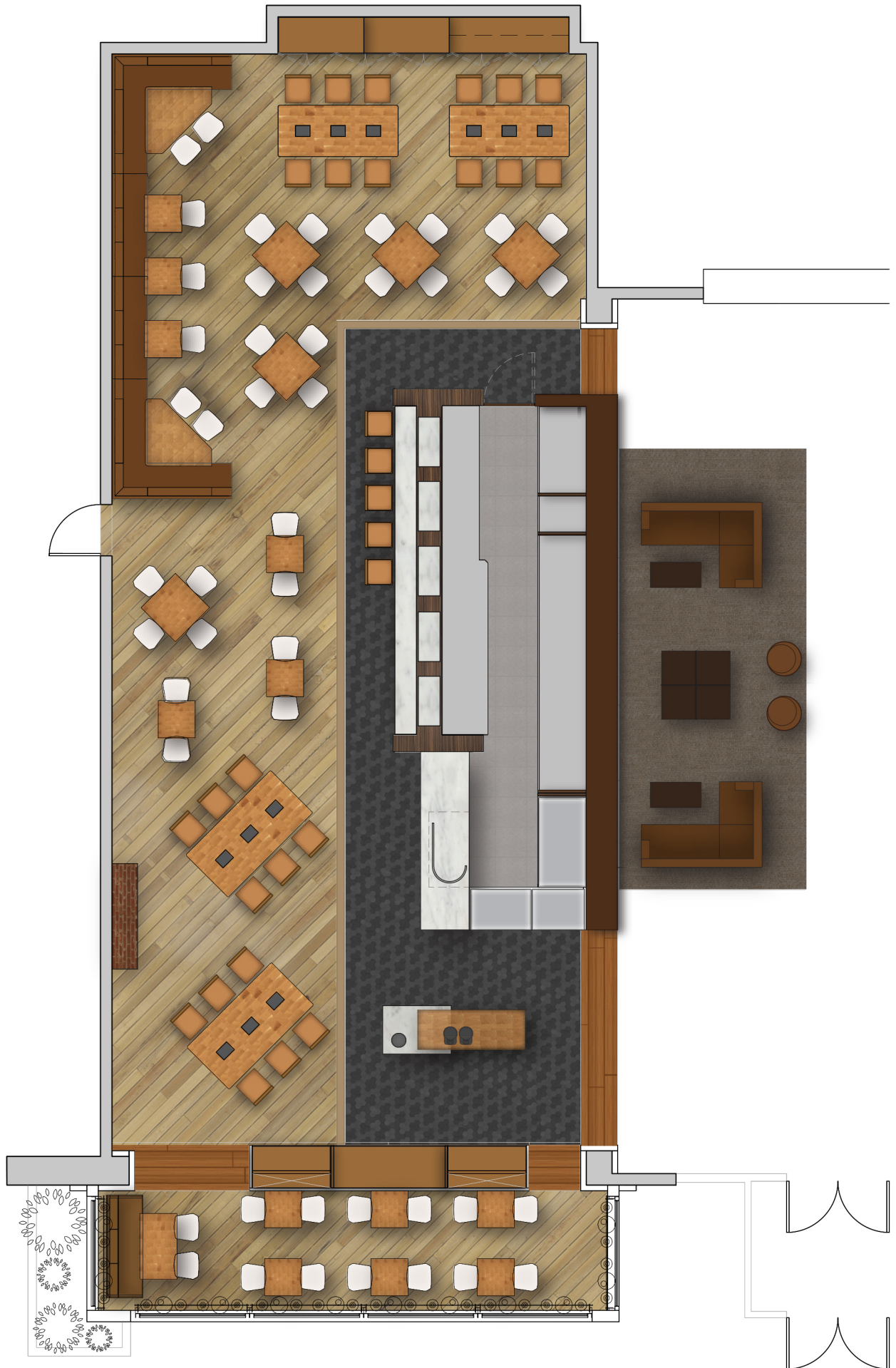
MARKET T1 FILTERED FLOORPLAN (W/ ADDITIONAL OPTIONS) | SCALE: 1/8" = 1'-0" SEATING COUNT: 77 + 12 ADDITIONAL AT BUFFET (NOT INCL. LIVING ROOM)
